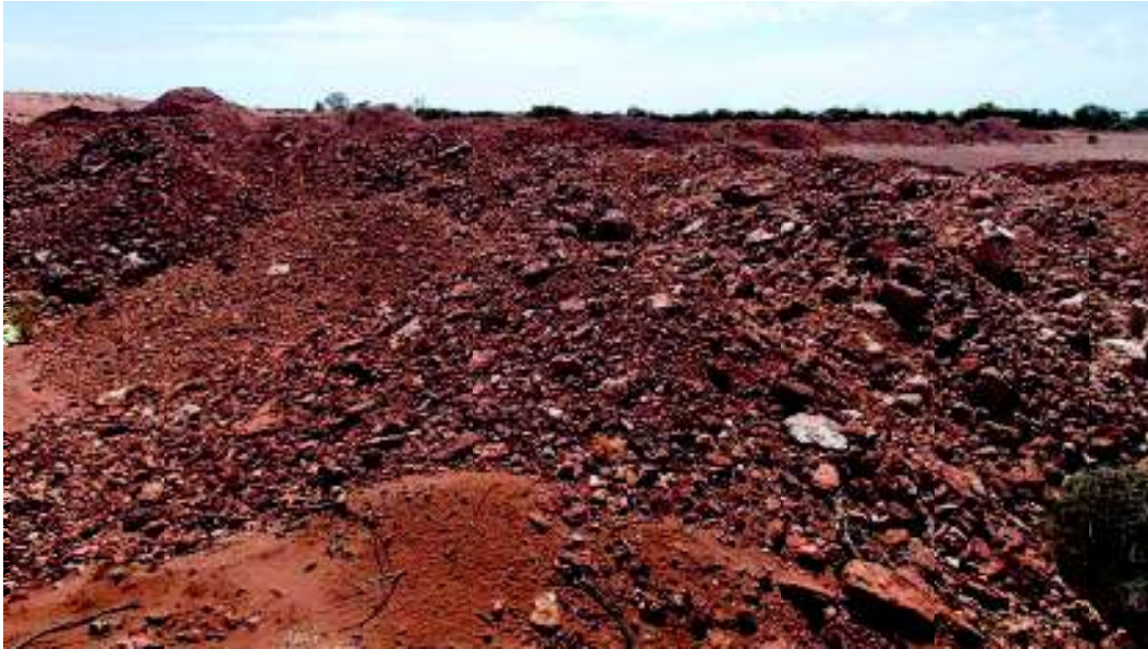
Figure 6. Mixed Calcrete/Gravel to be used as Fill, for creating the 15° slope or spread across the floor of the borrow pit
