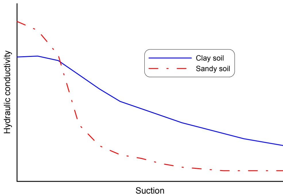
**Figure 4:** Representation of the variation of hydraulic conductivity with soil suction.
