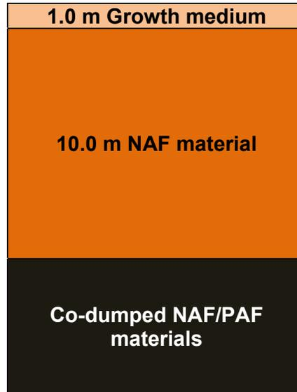
**Figure 2:** Current capping profile to be constructed at TGP.
