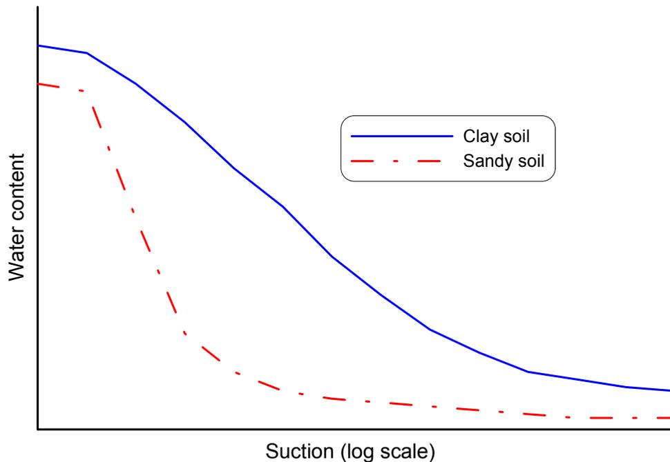
**Figure 3:** Relative patterns of soil water content vs. suction for sandy and clay soils.
