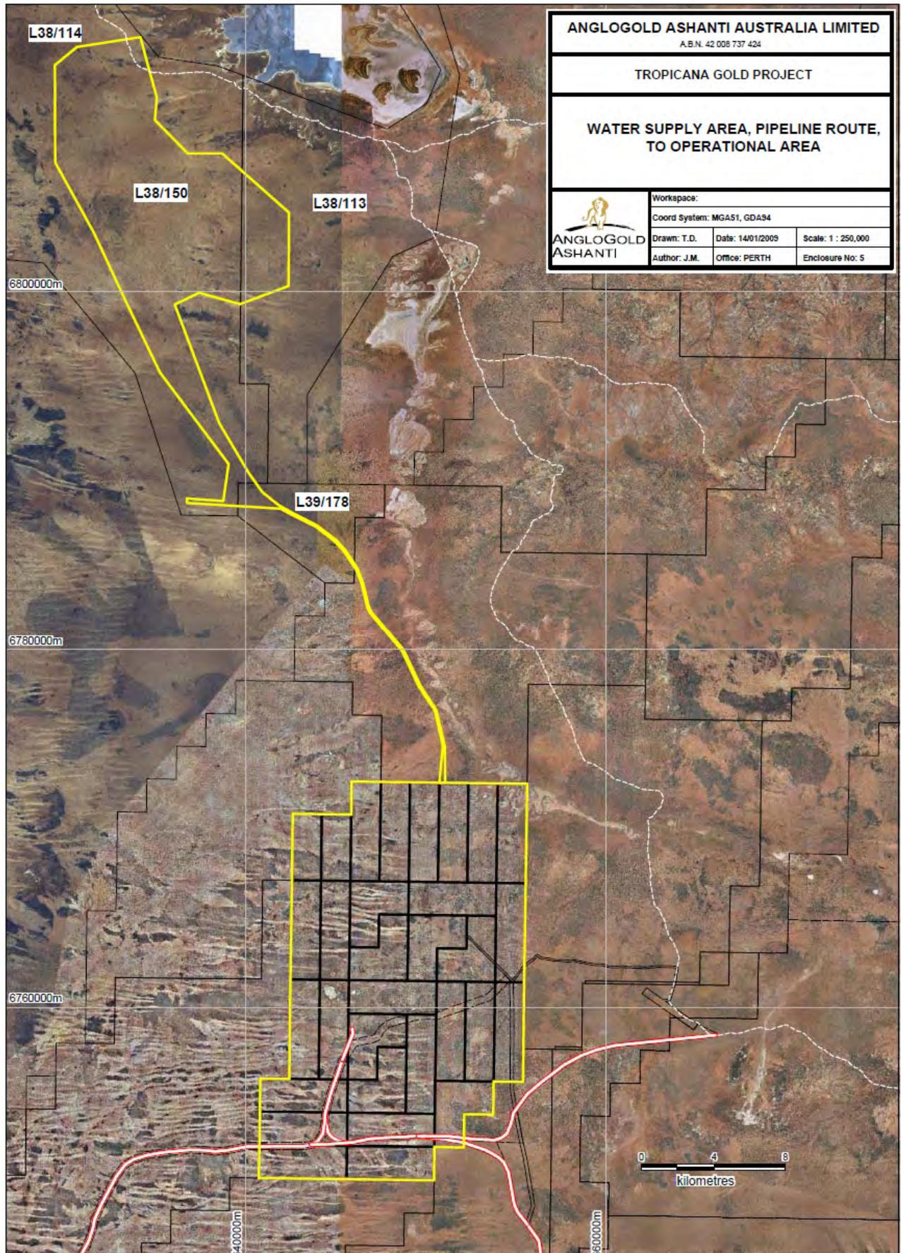
Figure 5: Minigwal Trough Water Supply Area & pipeline to Operational Area
