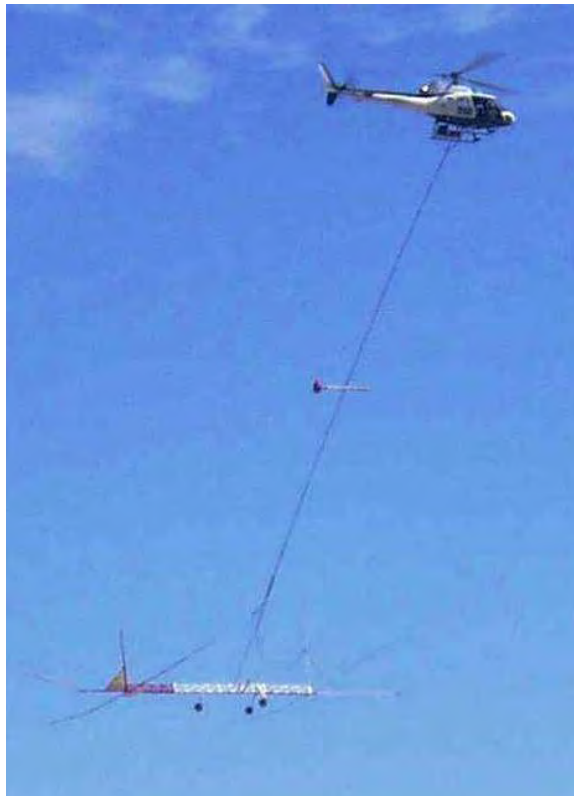
Figure 3-3: RepTEM survey showing magnetometer stinger and transmitter and receiver coils (hoist) slung 30m beneath the aircraft, and flown 30m above the land surface
